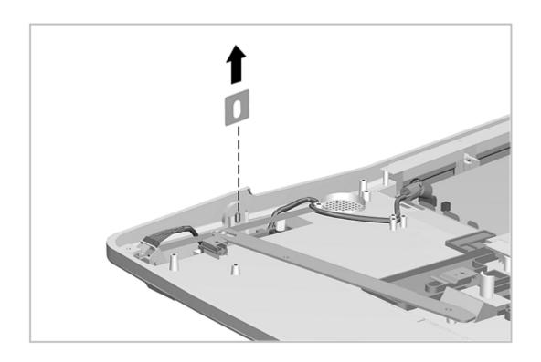
Figure 7-41. Removing the Security Lock Bracket
